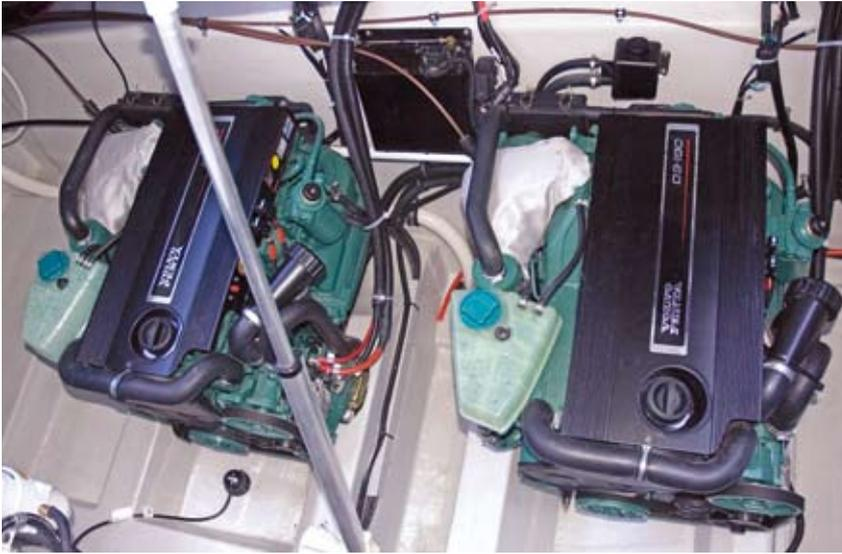
Twin 4.3-litre Volvo-Penta petrol engines are the recommended power package.
